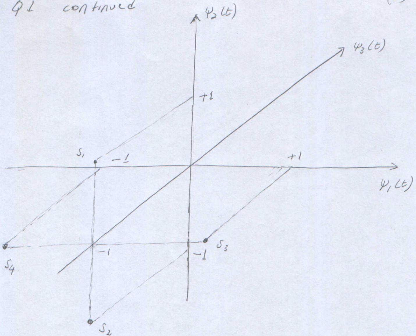
As seen, all vectors lie on the plane formed by  $\psi_1(t) - \psi_2(t)$ . The same can also be detected by examining  $s_1(t) -- s_4(t)$  or vectors  $s_1 -- s_4$  since in these  $\psi_3(t)$  is always present as  $-\psi_3(t)$ .
